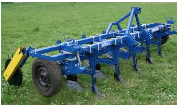
Figure 3. Device for soil modeling in interrupted furrows for weeding crops, simultaneously on 5 intervals, DMBC5-0
