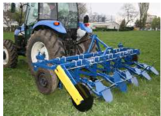
Figure 3. Device for soil modeling in interrupted furrows for weeding crops, simultaneously on 5 intervals, DMBC5-0
