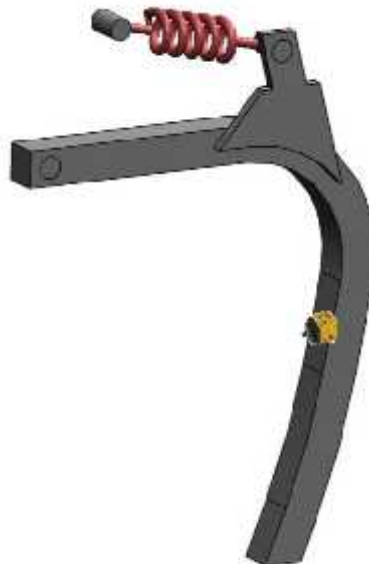
Fig.3 Vibratory working tool equipped with inclinometer
