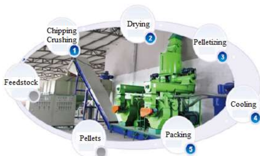
Figure 1: Stages of pellets production [10]
