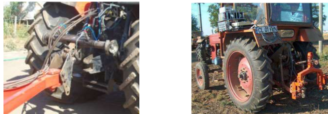
Figure 4. Drawbar / frame load cell mounted between tractor and towed machine [8]
