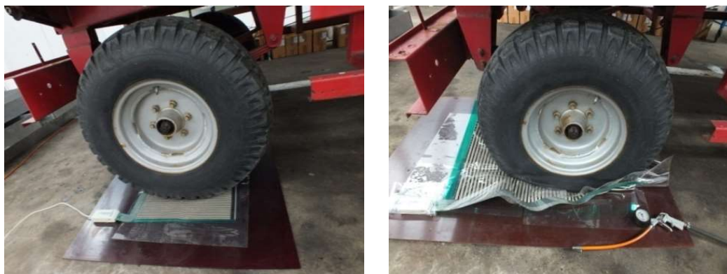
Figure 2: Testing with 21.18 kN wheel load, at tire inflation pressure of 300 kPa (left), respectively 180 kPa (right) [12]
