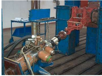
Figure 9. The mechanical testing of traction device type mounted on the stand [16]
