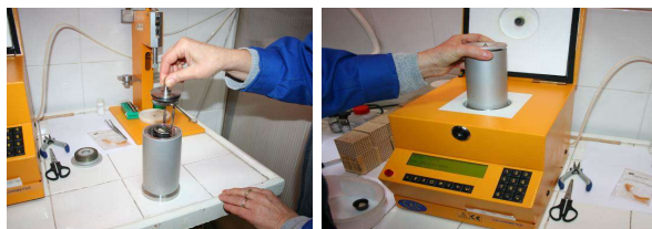
Figure 3: Determinining the calorific power for common agrimony briquettes
