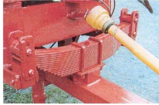
Figure 3. Drawbar with suspension mounted transversely in front of the trailer [7]
