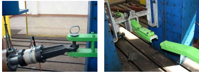
Figure 5. Fatigue testing of drawbar on HIDROPULS installation [13]
