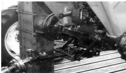
Figure 11. The mechanical testing of drawbar on the HIDROPULS stand [17]
