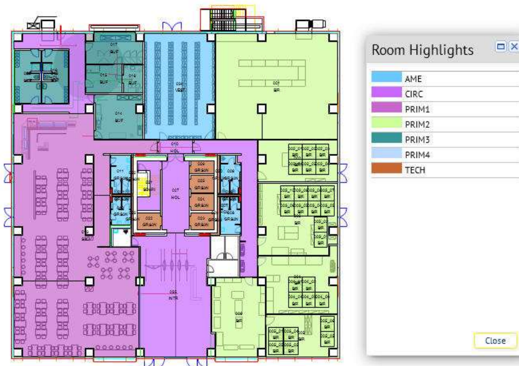
Figure 2: MultiGalaxy, ground floor, the functional structure of spaces according to EN 15221-6
