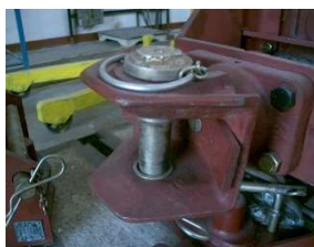
Figure 1. The coupling system tractor - trailer [4]
