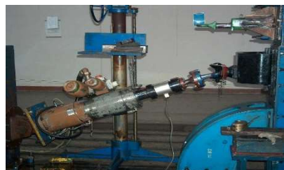
Figure 2. The coupling system in the testing device on the stand [4]
