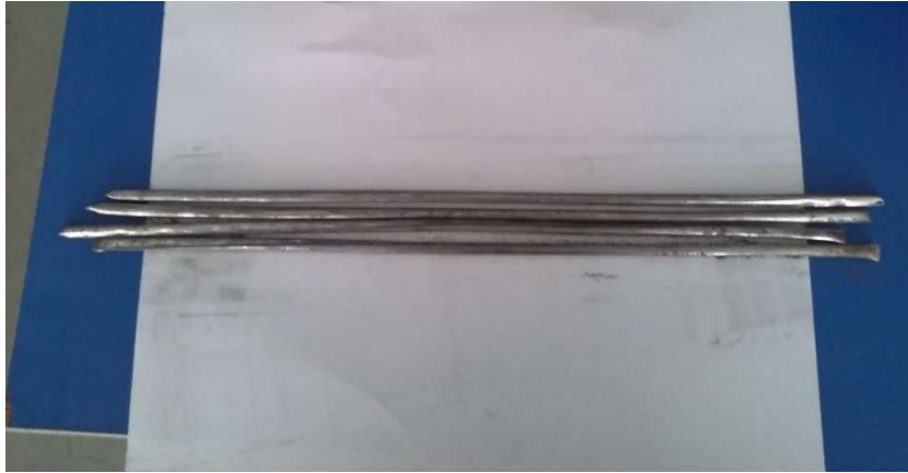
Figure 7. Experimental electrodes of the type steel with wolfram carbons core
