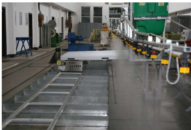
Figure 4: Stand for measuring the liquid distribution under a spray boom
