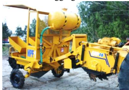
Figure 8: Multipurpose machinery: working soil, seedlings planting, seedlings watering
