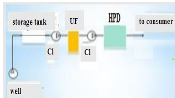
Figure 1 – Technologic scheme of Water treatment installation.
