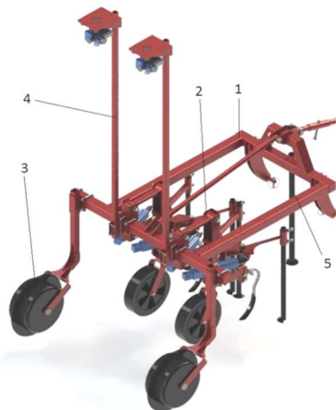
Figure 4: Technical multifunctional equipment designed to mechanical maintenance in row and between crop plants
