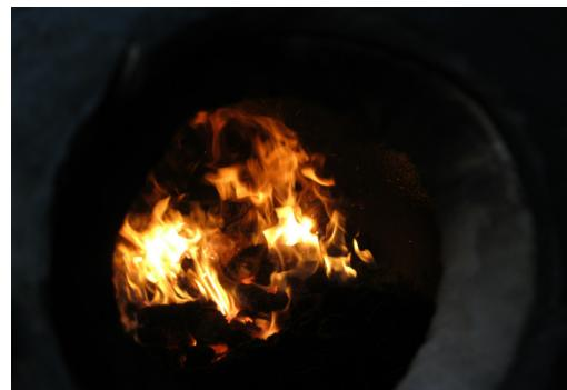
Fig.7. Aspect of briquettes burning in the flame tube
