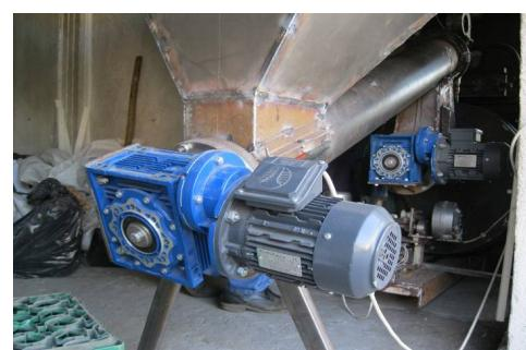
Fig.6. Details from the automated briquette feed system
