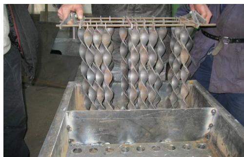
Fig.5. Flue tubes cleaning equipment
