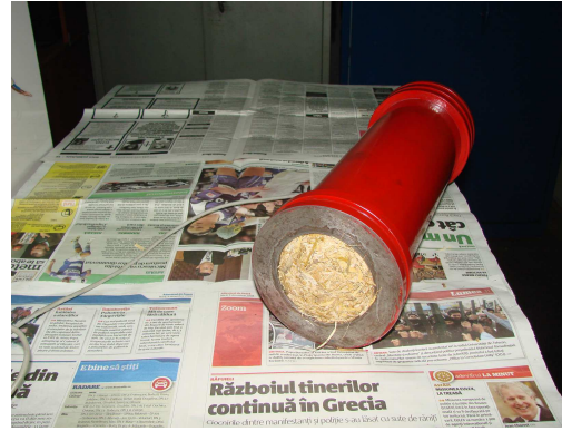
Fig.2 Briquette in the pressing cylinder it is shown how the material is felting
