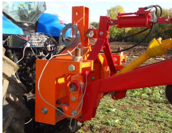
Figure 2: The frame with strain gauge marks, coupled to three-point linkages 3 category according to ISO 730:2009
