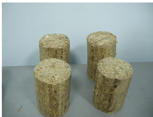
Fig.5 Maize stalks briquettes obtained on the sawdust presses by changing the operational drive
