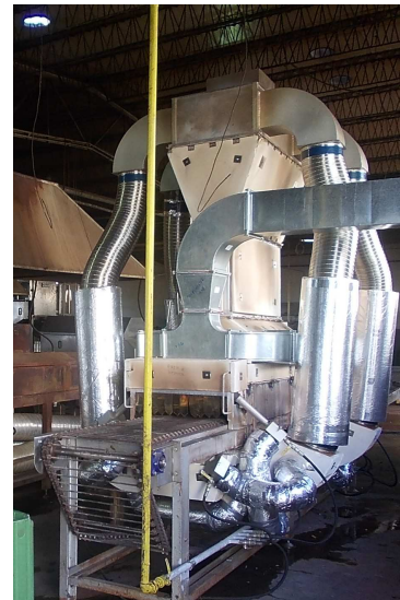
Fig. 4. A picture of the heat recovery solution with the ejector
