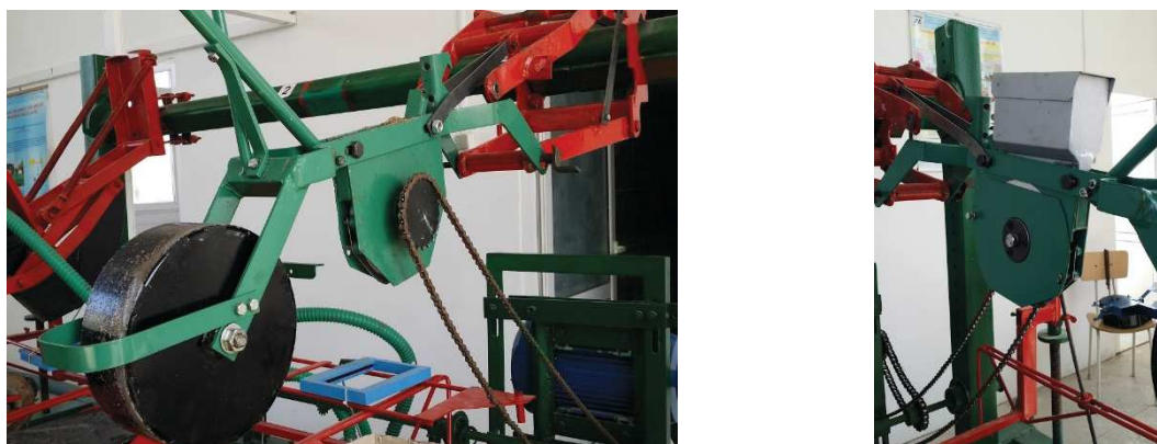
Figure 4: The sowing station of SMP-0 equipment fitted on stand
