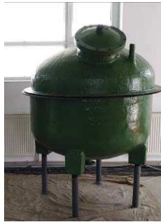
Figure 3: Digester for wet anaerobic digestion process
