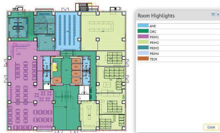
Fig. 3. MultiGalaxy building, ground floor, functional structure of spaces according to EN 15221-6
