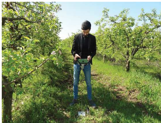
Figure 1: Electronic penetrometer with digital display Eijkelkamp Penetrologger equipped with a humidity sensor Eijkelkamp Thetaprobe
