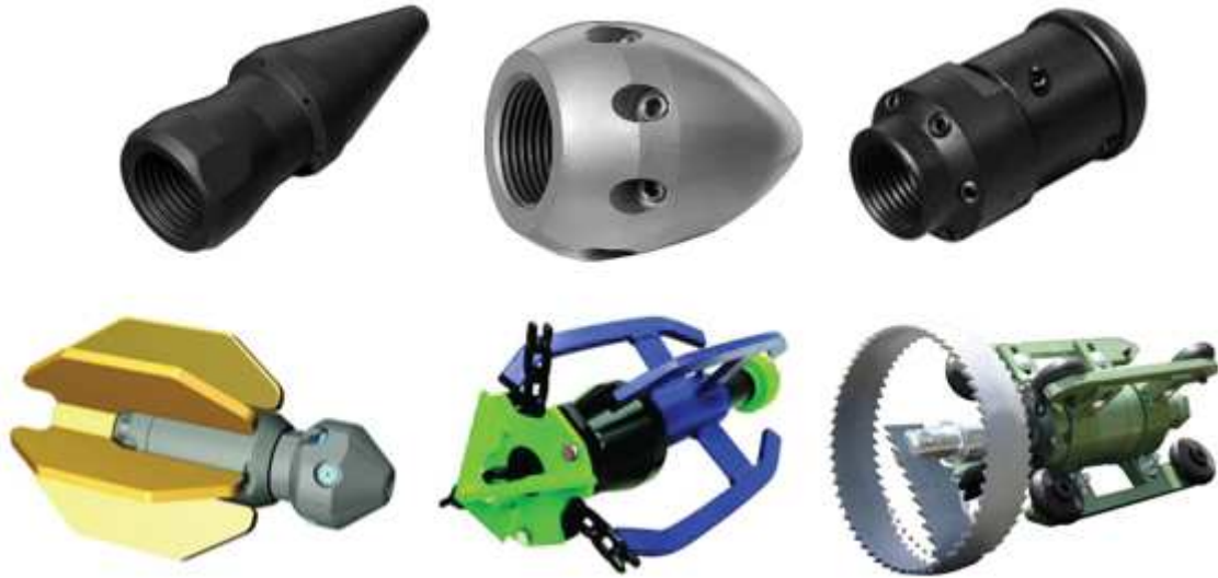
Fig.6. Various types of cleaning devices for sewers and waste water channels, [10]: general cleaning and obstacle penetration device; frontal and six side nozzles that can be replaced, used for greases; rotary head device (6 nozzles at 30° and 3 nozzles at 60°) for greases; rotary head device with forward nozzles in the rear body; device with nozzles and impact chains for strong agglomerations and roots; saw blade device for cutting roots.
