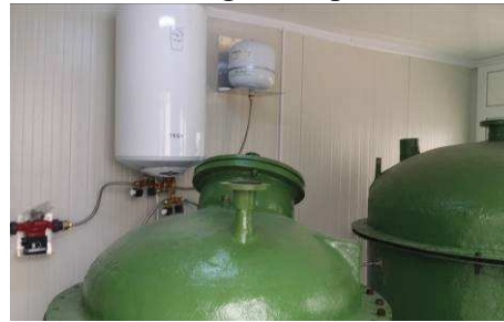
Figure 2: Digester for dry anaerobic digestion process
