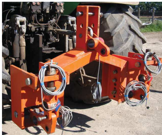
Figure 2: Device with tensometric transducers (tensometric frame)
