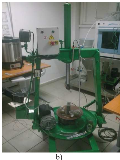
Further, the oil products were pressed, using for this purpose a laboratory mini-press (fig. 3a), attached to a big hydraulic press (fig. 3b).
