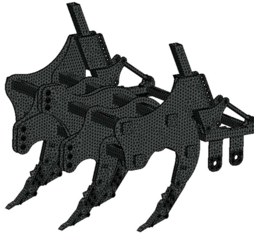
Figure 7: Structure discretization: Projection of finite elements on the structure border
