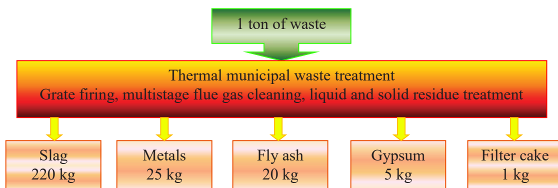
Figure 5: Mass balance for solid residues from a grate incineration plant [13]
