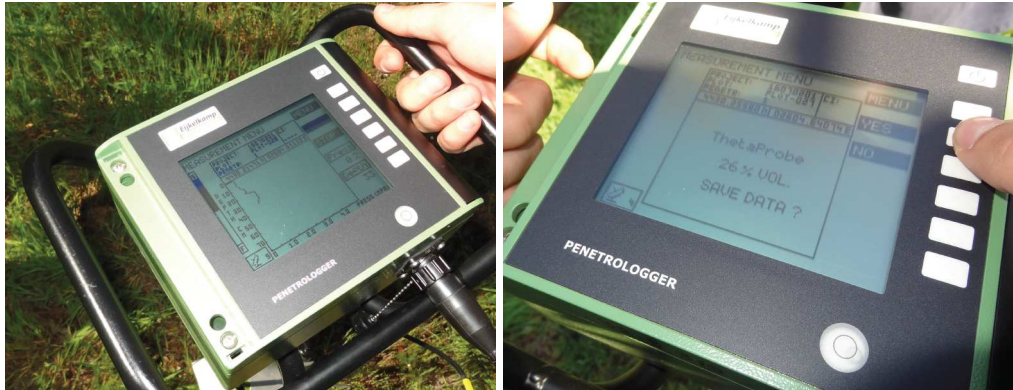
Figure 2: Measurement of press pressure and local humidity
