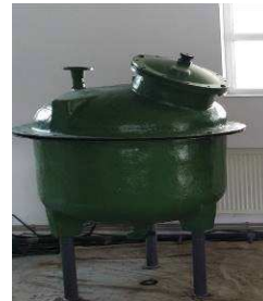
Figure 2: Digester for dry anaerobic digestion process
