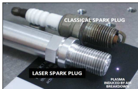
Figure 1: A photo of a laser spark plug is shown in comparison with a classical spark plug. The plasma induced in air by optical breakdown is visible. (Courtesy of INFLPR, Laboratory of Solid-State Quantum Electronics, Magurele, Romania).
