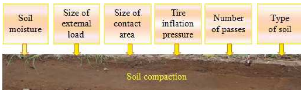
Figure 2: Main factors that influence the artificial compaction of soil
