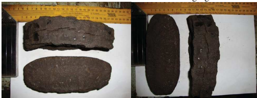
Figure 6: General view and dimension of peat briquettes
