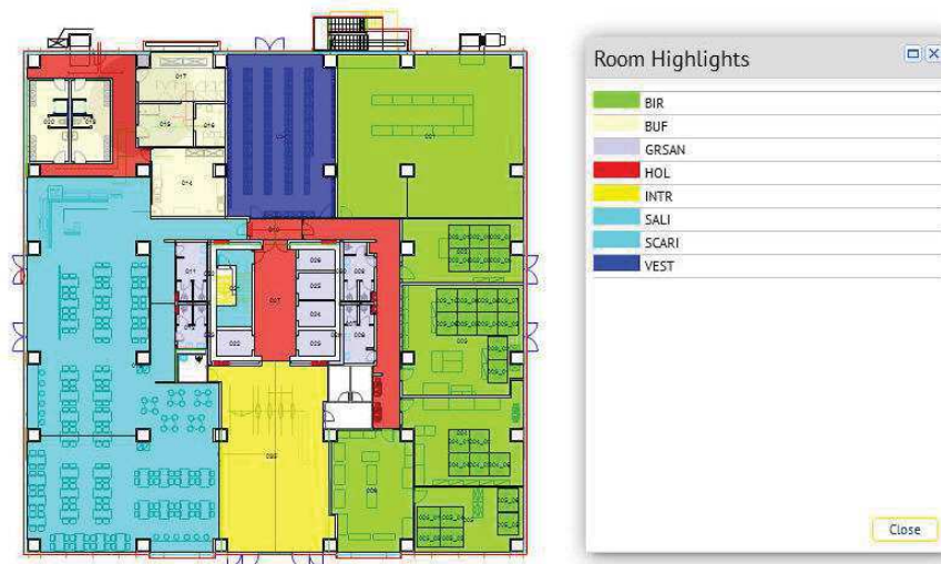
Fig. 4. MultiGalaxy building, ground floor, space structure according to SR 1907-2
