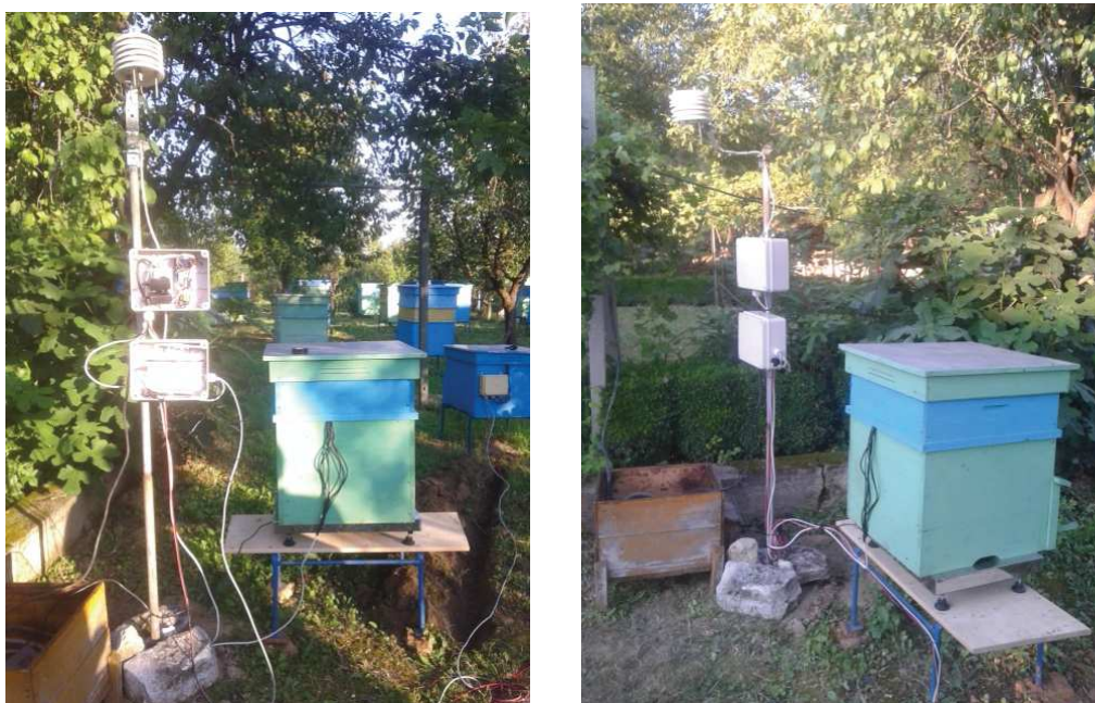
Fig.1. Meteorological station for measuring the microclimate in the bee colony and beyond
