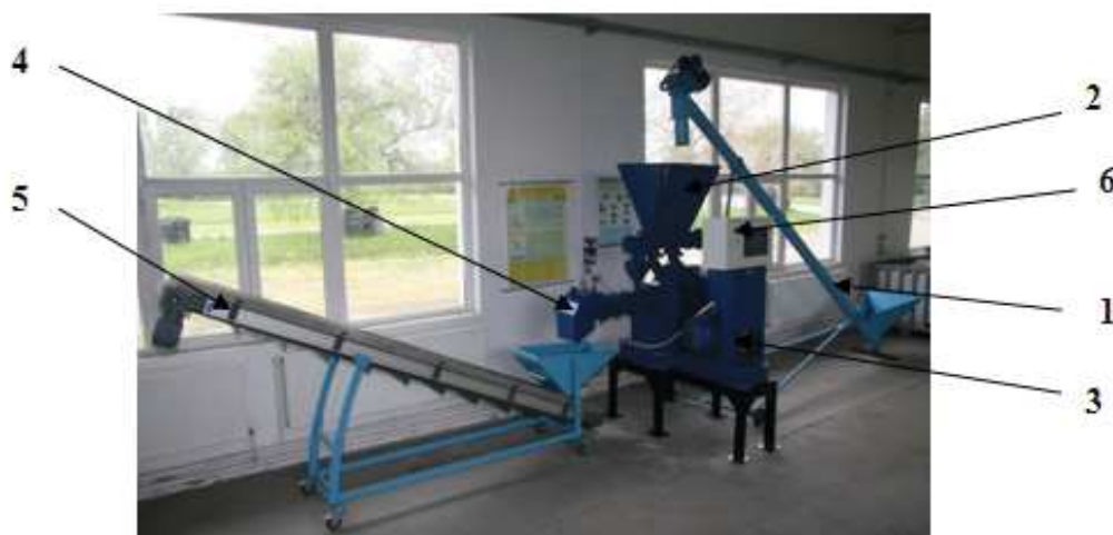
Figure 1: Installation for soybean seeds superior capitalization – IVSS / INMA Bucharest
