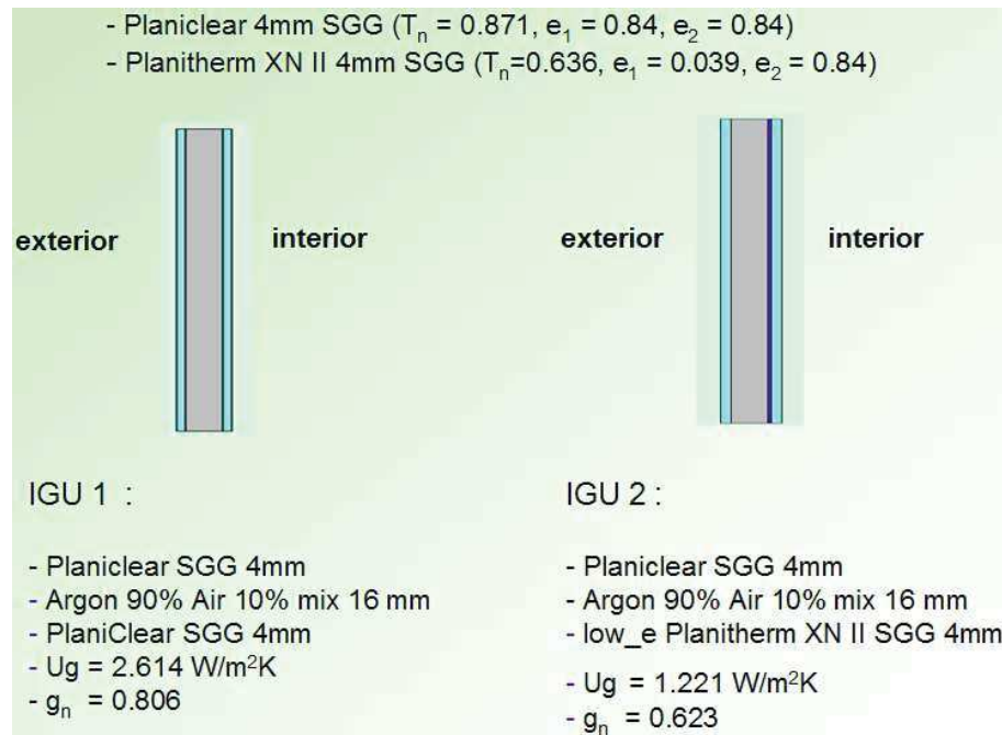
Fig. 2 The two IGUs made of SGG glass panes, Planiclear and Planitherm XN II
