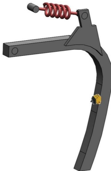
Fig.3 Vibratory working tool equipped with inclinometer
