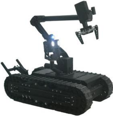
Fig. 3 The rescue robot HD2 - “Mastiff” developed by the SDR Tactical (Photo: sdr tactical.com)
