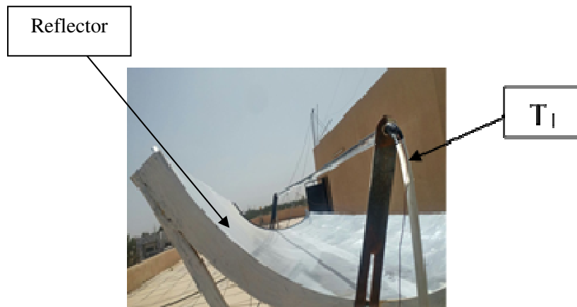
Figure 1. Experiment parabolic trough solar with the receiver
