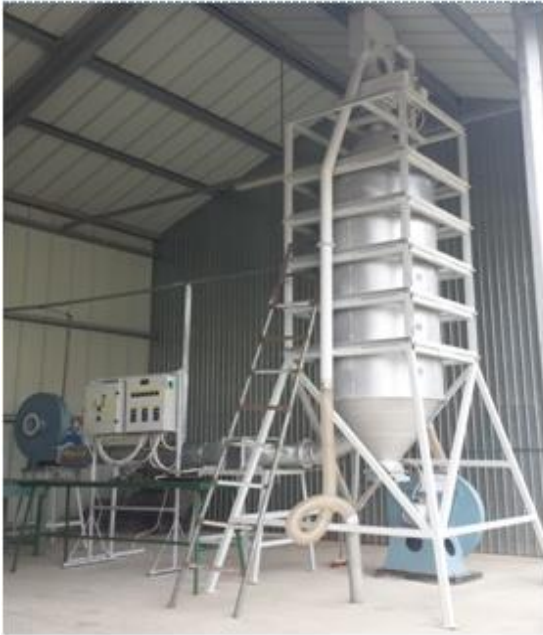
Figure 7: Innovation vertical drier with heat recovery
